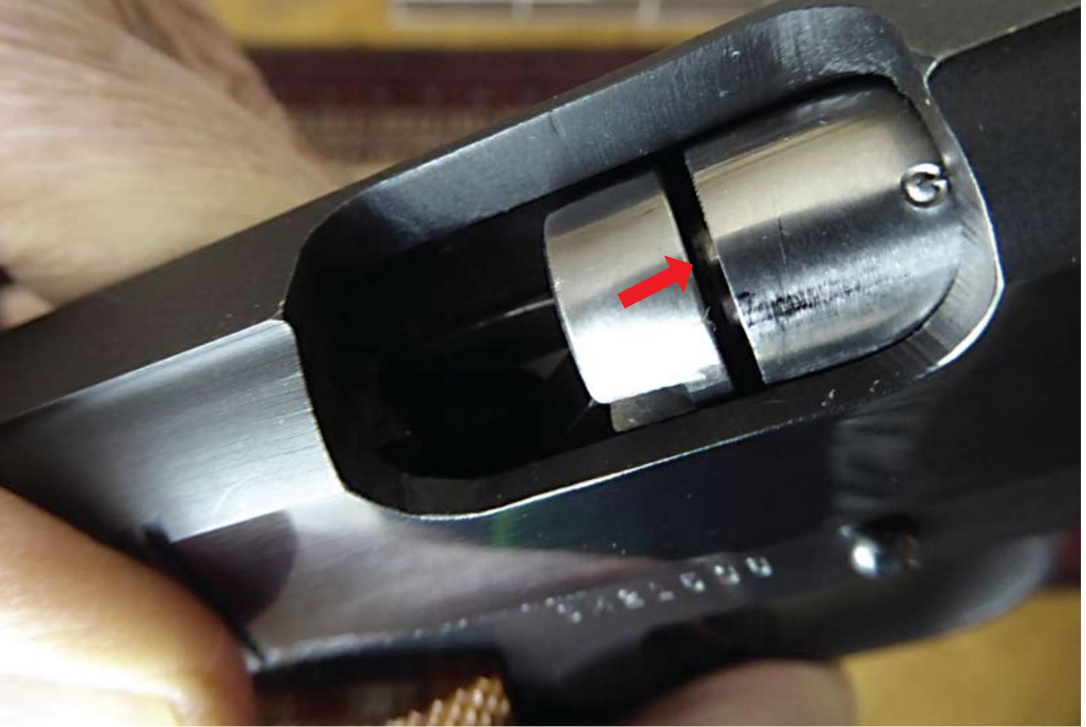
*Floating chamber in maximal hinterer Stellung (schwarzer Spalt)*
